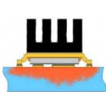
⑦ Mounted to a PCB with a thin gap filler and heat sink. (still air)
